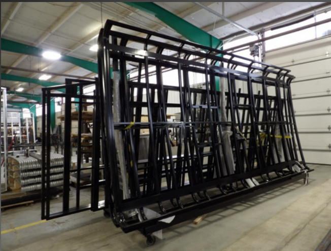
~ Powdercoated steel walls, roof and stepwell ~
