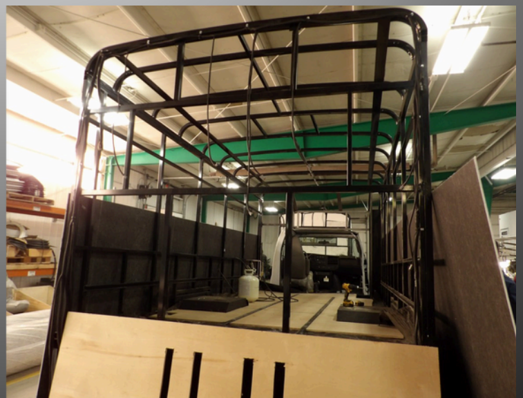
~ 3/4" marine plywood flooring ~
