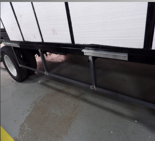
~ Welded skirts with FRP panels ~
